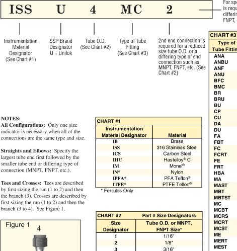
For special application tees, a 3rd end connection is required for a reduced size tube 0.D. or a differing type of end connection such as MNPT, FNPT, etc. (See Chart #2)
