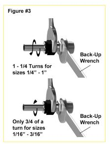
Note: For all sizes, tighten plugs (P), machined ferrule end of port connector (PC) and the **Unilok** end of the Female AN Adapter (ANF) only **1/4** of a turn.
