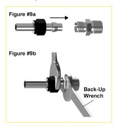
NOTE: To extend the life of a presetting tool, lubricate the tool with a lubricant compatible with the system's tubing material, environment and media. Also, at times, an oversized or very soft tubing may tend to stick in the pre-setting tool after make up. To remove the tubing, gently rock the tube back and forth. Never turn the tube with pliers or another tool, as such action may damage the sealing surfaces.
