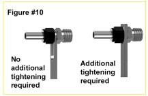
3. If the Gap Gage will not enter between the fitting's nut and body hex, no additional tightening is required.
