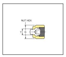
Plugs are used to plug an unused port of a Unilok tube fitting.
