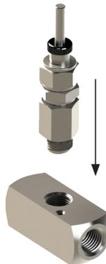
12. Place the bonnet lock back over the body and align slot with the threaded socket screw hole.
