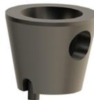
10. Position the plug seat over the body so that the pin aligns with the pin hole in the orifice of the body. Push the plug seat into the body and the pin should fit into the pin hole. This prevents the plug seat from rotation
